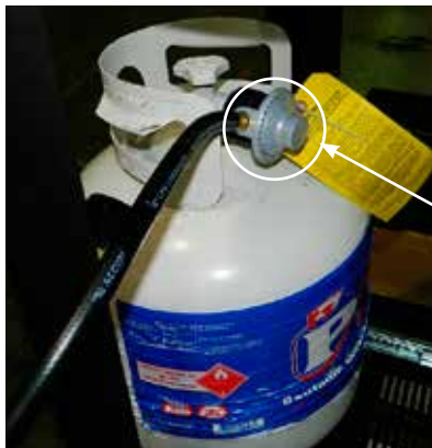
Gas connection @ tank
